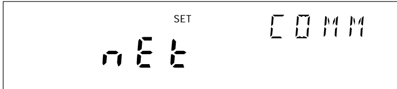
Communications display for setting the network type
