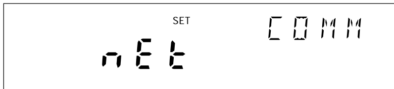
Communications display for setting the network type
